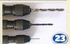
These are the three pin vices and drill bits I used in preparing the headlamps to be fitted with LEDs. Bit sizes are: top 2.0mm, middle 1.5mm and bottom 0.6mm.
