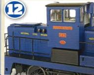
next stage, fitting a cab light requires access to the interior, shown hen with the chassis in situ. Release all the handrail to cab push-fit connections before pulling the cab moulding upwards
