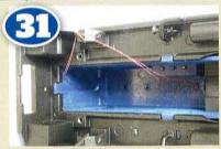
The wires from the front lamp and the cab light can be seen here. Each single strand wire was soldered to an appropriately coloured insulated wire and then fixed in place with cyano adhesive to prevent accidental damage. Insulated wire is much more robust so this was used as the flexible connection to the decoder.
