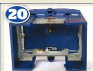
By carefully prising the centre of the glazing strip I was able to feed a DCC Concepts wired 'Nano LED' through the channel which I fixed with cyano adhesive to the roof.
