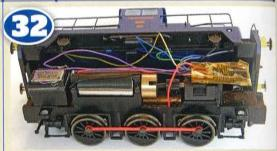
Having removed the rear extension of the motor bracket to create space to fit a stay alive capacitor which I then found to be un-necessary, I fitted a larger speaker to the rear. There is sufficient space next to the decoder to fit a capacitor or a second speaker in future. The final connections for the lighting consist of yellow to one lamp, white to the other, green to the cab light and blue for the common return.
