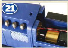
To provide clearance for the single strand lacquered wires I cut a notch in the mating channel at the rear of the forward engine room - compare with Step 13.
