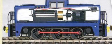
The superstructure is fixed to the chassis with four screws, two of which can be seen next to the brake rigging at each end of the chassis. The couplings pass through each buffer beam, so must be removed before the body can be lifted dear.
