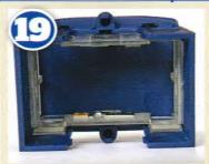
With the moulding removed, the inner roof can be seen. Note the end of a rectangular section channel in the cab bulkhead next to the glazing.
